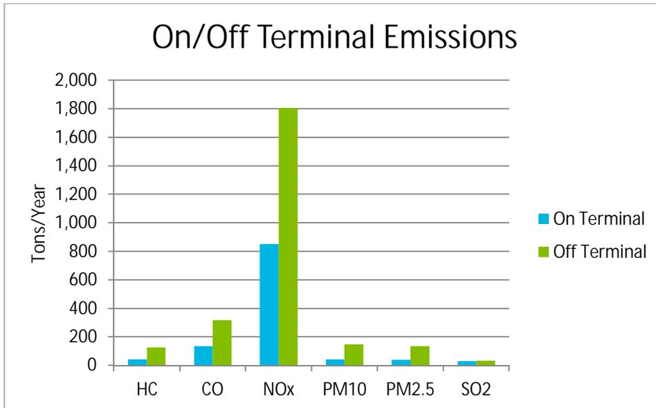
**Figure 2-7: Comparison of Emissions Inside and Outside of Terminal Boudaries**
